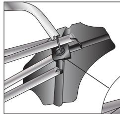
Notch in kickstand lines up with rib on back hub to lock kickstand in place.
